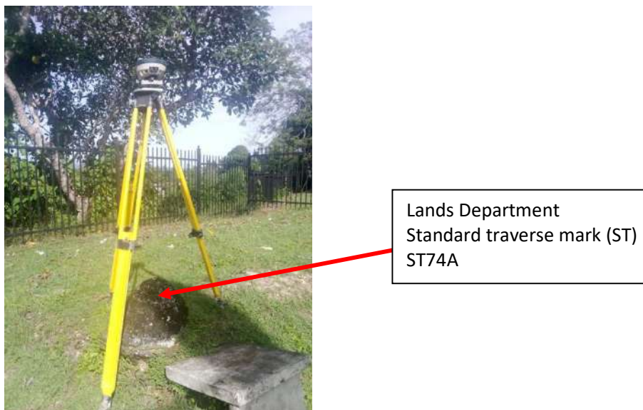
Figure 3.0: Survey mark of Origin ST74A
