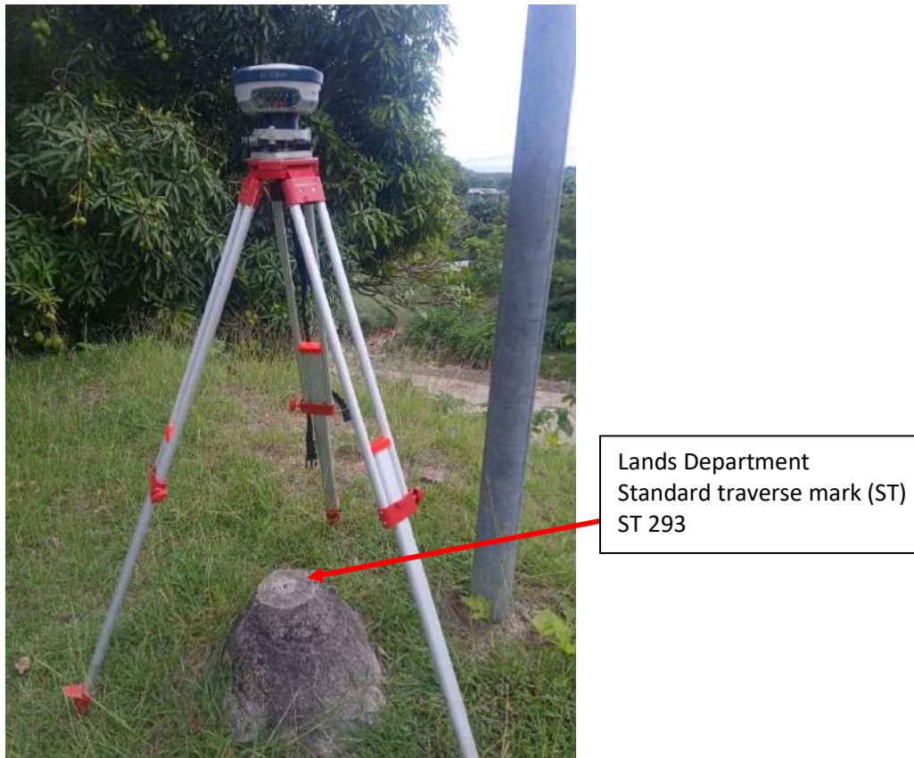
Figure 3.0: Survey mark of Origin ST 293
